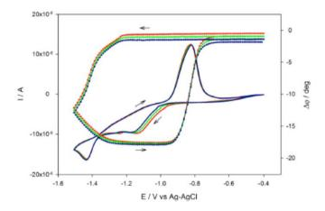
Figure on the left shows the current and phase-shift monitoring when potential step of -1.3V is applied. With this potential step below the Nernst equilibrium potential only few layers of cobalt are deposited on the HFF-QCM gold electrode. The potential is maintained during 30 seconds and a linear potential decrement with a rate of 10mV/s is applied. Phase-shifts show the deposition and dissolution of cobalt during the experiment.
