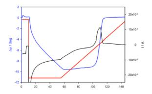
Figure on the left shows the current and phase- shift monitoring when potential step of -1.3V is applied. With this potential step below the Nernst equilibrium potential only few layers of cobalt are deposited on the HFFQCM gold electrode. The potential is maintained during 30 seconds and a linear potential decrement with a rate of 10 mV/s is applied. Phase- shifts show the deposition and dissolution of cobalt during the experiment.
