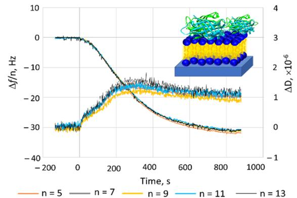
**Figure 4. Binding of streptavidin to biotinylated lipid bilayers. Note the maximum in the dissipation signal. The inset shows, schematically, two streptavidin molecules bound to the bilayer, to illustrate that the size of the streptavidin molecules is comparable.**
