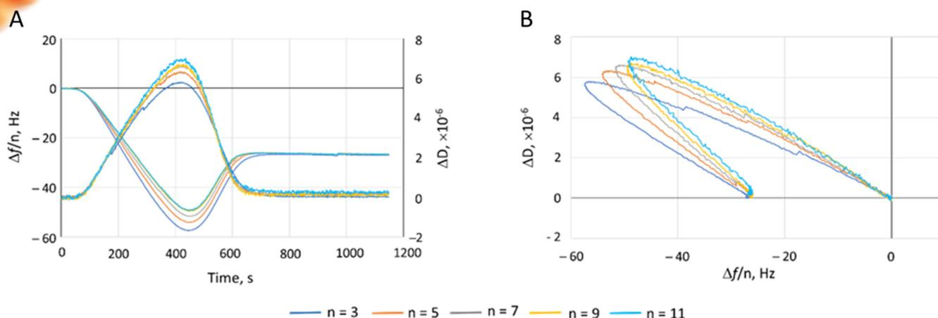
**Figure 2. A typical SLB formation experiment performed with a 5 MHz SiO<sub>2</sub>-coated sensor and 50 nm extruded DOPC liposomes in a 10 mM HEPES buffer pH 7.4 containing 150 mM NaCl and 2 mM CaCl<sub>2</sub>. (A) Frequency and dissipation vs. time. (B) Dissipation plotted as a function of frequency. Data for  $n = 1$  and  $n = 13$  are not shown.**
