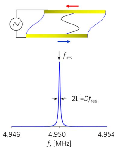
**Figure 2.** Top: A quartz resonator oscillating in a thickness-shear mode at the fundamental ( $n = 1$ , blue) and at the 3<sup>rd</sup> overtone ( $n = 3$ , black). The two surfaces move in the opposite directions, as indicated with the red and blue arrows. Gold electrodes are shown in yellow.
