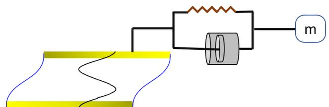
**Figure 7:** QCMD can be thought of sensing a force applied to the surface of a resonator. Applied force can be thought of as a mass  $m$  coupled to the resonator surface through a spring with a constant  $k$  (brown) and a dashpot that describes dissipative losses (in the simplest case, viscosity,  $i2\pi f\eta$ , grey).
