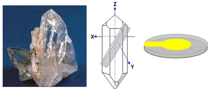
**Figure 1.** At the heart of QCMD is a resonator (right) made of a piezoelectric material such as quartz (left), cut at a certain angle relative to the crystallographic axis (middle). Electrodes deposited on the sensor surface are shown in yellow.
