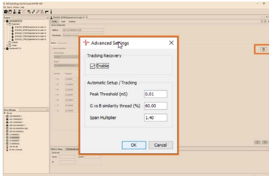
Figure 1. Tracking recovery setup panel included in AWS Suite software GUI.
