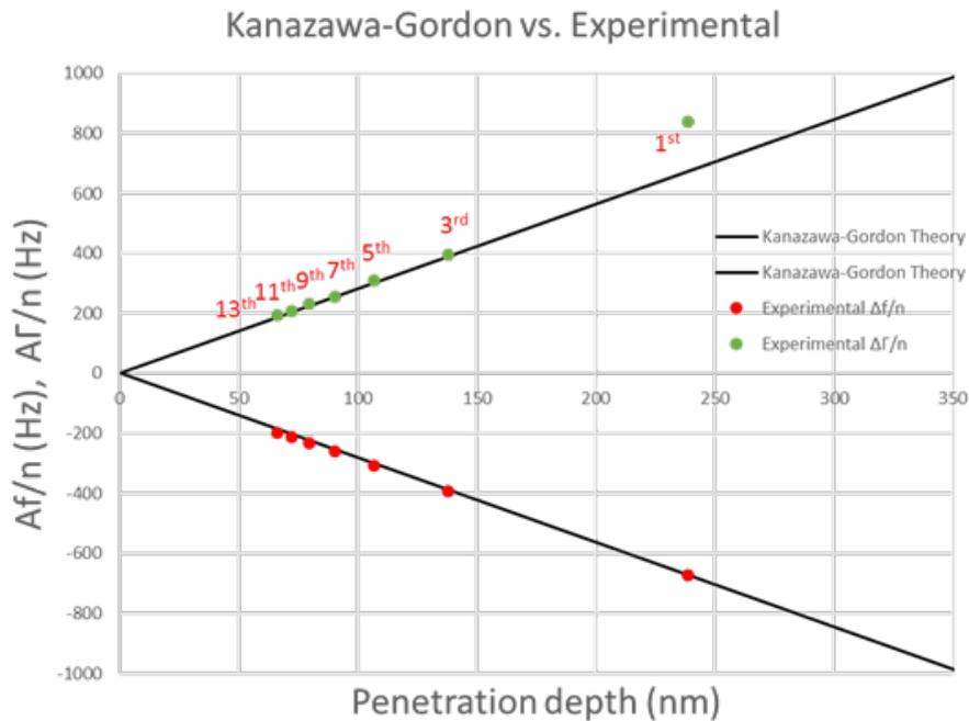
Figure 4. Kanazawa-Gordon equation prediction vs. experimental results.
