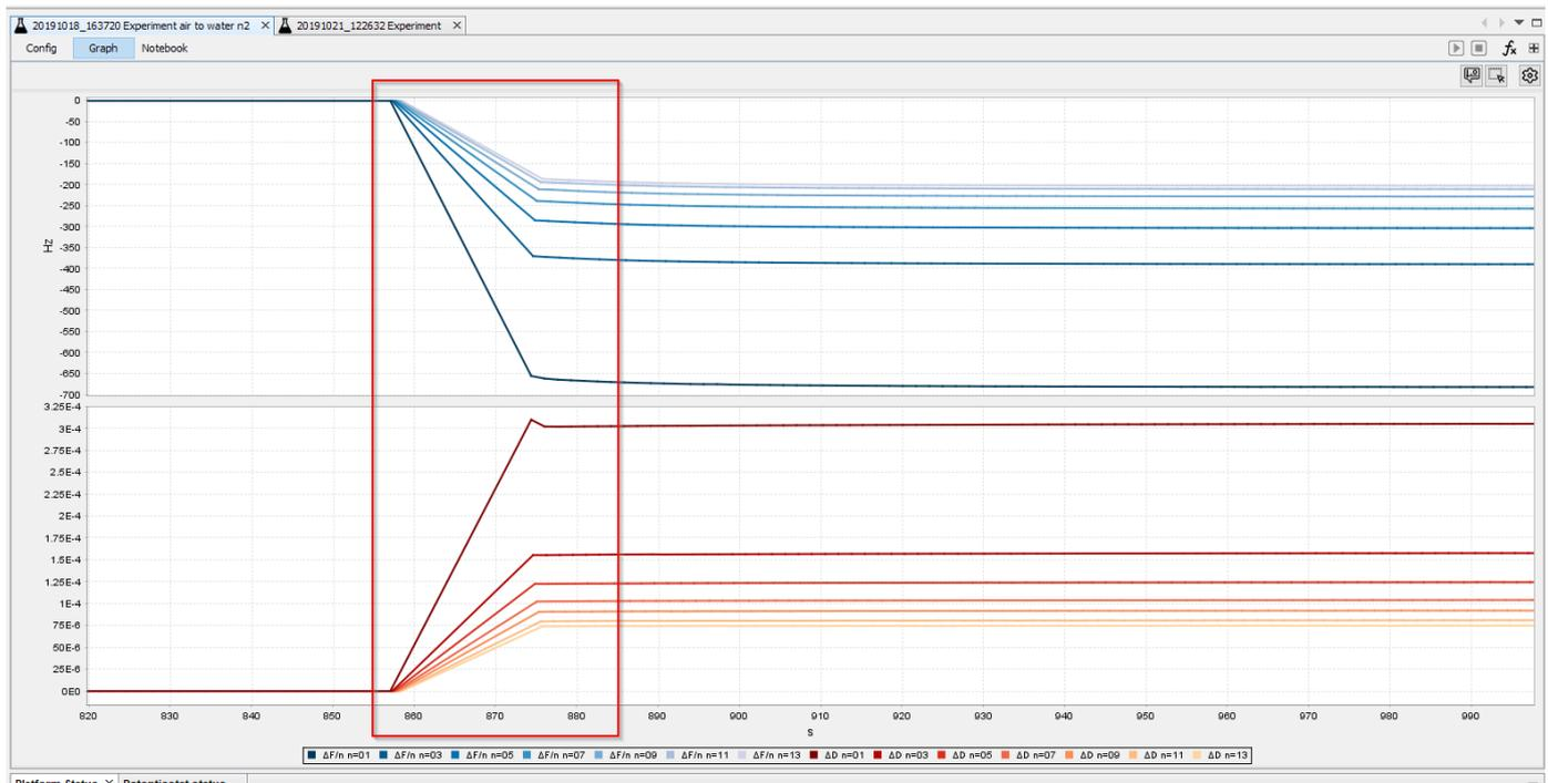
**Figure 3.** AWS Suite software GUI showing data gathered during one of the air-to-water medium exchange experiments. Blue curves represent the resonant frequency while red curves represent Dissipation. The red box shows the experiment part where the Tracking Recovery feature is run.
