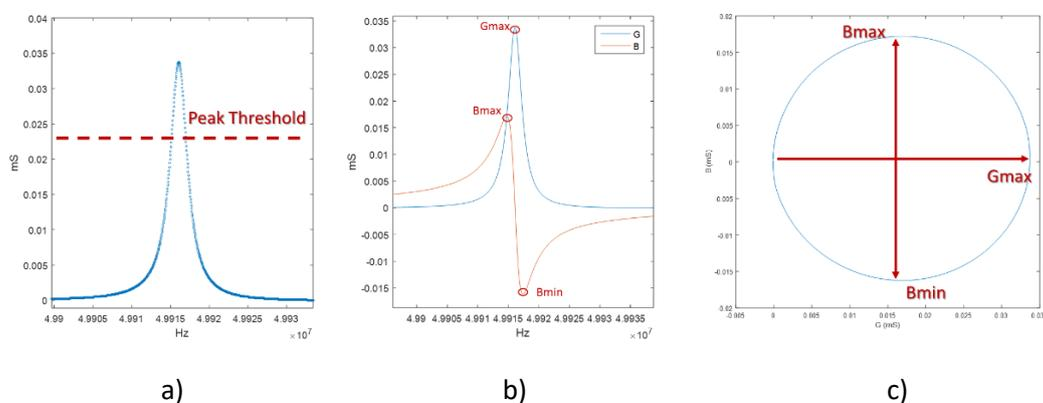
Figure 2. a) Diagram showing conductance spectrum and peak threshold. b) Diagram showing both conductance and susceptance spectra. Conductance maximum (Gmax), Susceptance maximum (Bmax) and susceptance minimum (Bmin) have been marked. c) Diagram showing Susceptance versus Conductance similarity relation.
