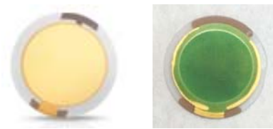
Figure 9: A QCMD sensor before and after the aniline polymerization.
