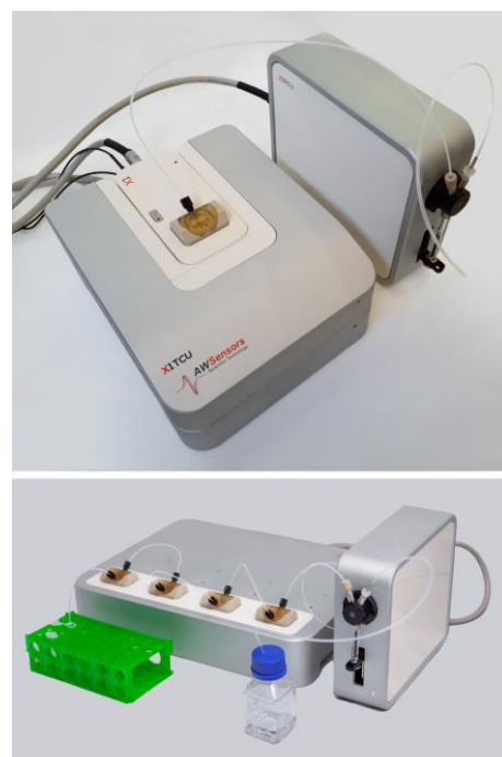
Figure 1: AWSensors single-channel (X1) and 4-channel (X4) advanced QCMD instruments with Flow Control Units (FCUs).
